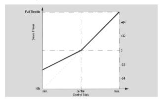
This diagram shows adjustments often encountered in practical use. The hover point has been selected as "point". A "G" of 50% results in the throttle servo being markedly slaved by the throttle / pitch control below the hover point.
