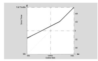
For this example, the take -over point has been moved upward, while "G" remains unchanged. The diagram illustrates that throttle preset now affects the hover flight region, a condition which should normally be avoided.
