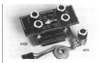
the PROFITRIM-Module (Part No. 4109) is available as special equipment, which permits adjusting the primary functions in a common manner by rotary controls (regulators). The module is installed into one of the upper module stations of the transmitter case and features four regulators for the functions:
