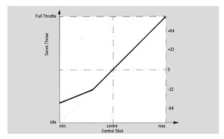
Here "G" has been left un changed, while the take -over point has been moved farther down (-32). The diagram makes clear that the initial value for the carburettor opening has been lowered, due to "G" being retained at 50%. The slope of the curve in the lower region remains unchange d.
