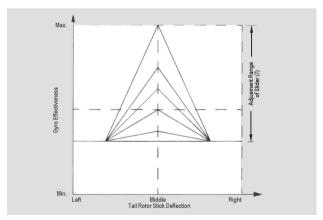
Here too, minimum gyro effectiveness is obtain at 60% of the control stick deflection, however, the value is not 0 as (in example 3), but corresponds to the adjustment of regulator 1 at the gyro sensor.
