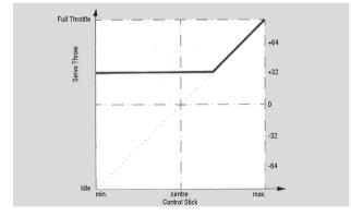
This last diagram shows the effect of moving the take -over point upward. It demonstrates that here too, marked rise of hover RPM will have to be achieved, which can not be stable as no load-dependent tuning is performed. This kind of adjustment may only be switched on for some of the aerobatic manoeuvres to avoid unwanted loss of RPM in inverted flight with the pitch reduc ed markedly, if at all.
