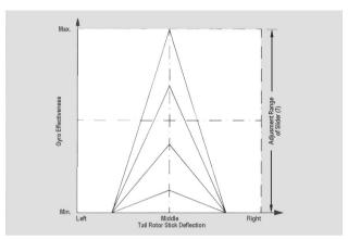
Unlike example 1, complete fading has occurred by 60% of tail rotor control stick deflection.
