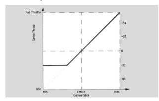
When the take-over point is displaced downward, the diagram above results. The throttle servo is slaved here to a point far below the hover point.
