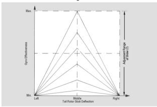
Gyro effectiveness can be infinitely variably adjusted from 0 up to maximum by slider 7. Actuation of the tail rotor control results in linear fading of gyro effectiveness with value 0 reached at the control stick end points.
