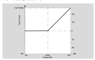
In this example, the take -over point is returned to the hover flight point again (point = 0). With "G" set at 100%, a genuine power on approach effect results, which is to say that the servo will hold a constant value below the take -over point, while being slaved in the normal way by the throttle / pitch control above it. This kind of throttle preset is useable, e.g. for throttle p reset (2) hover manoeuvres of the FAI competition programme described earlier.
