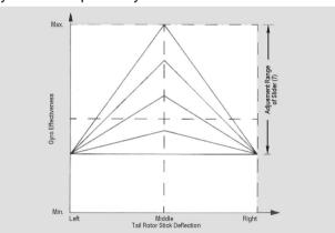
The gyro effectiveness can be varied between the two adjusted values by slider 7, but can not be reduced to 0. Automatic fading by the code 67 mixer is also effective only down to the value set be regulator 1.
