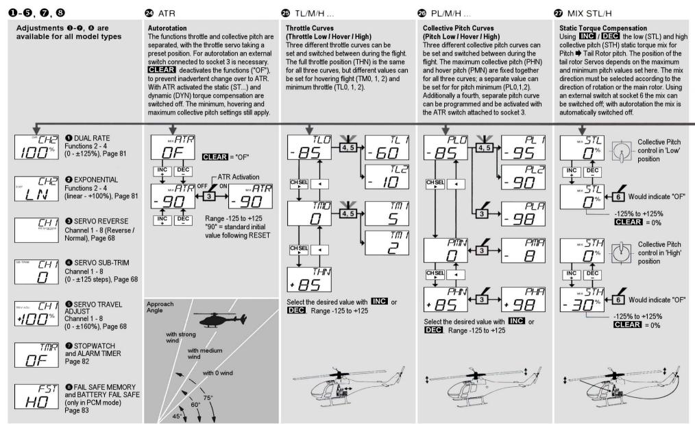
All mixer data can be set to 0, i.e. switched off using the CLEAR key. Display "OF" = the external mixer is switched off. 64 Helicopter
