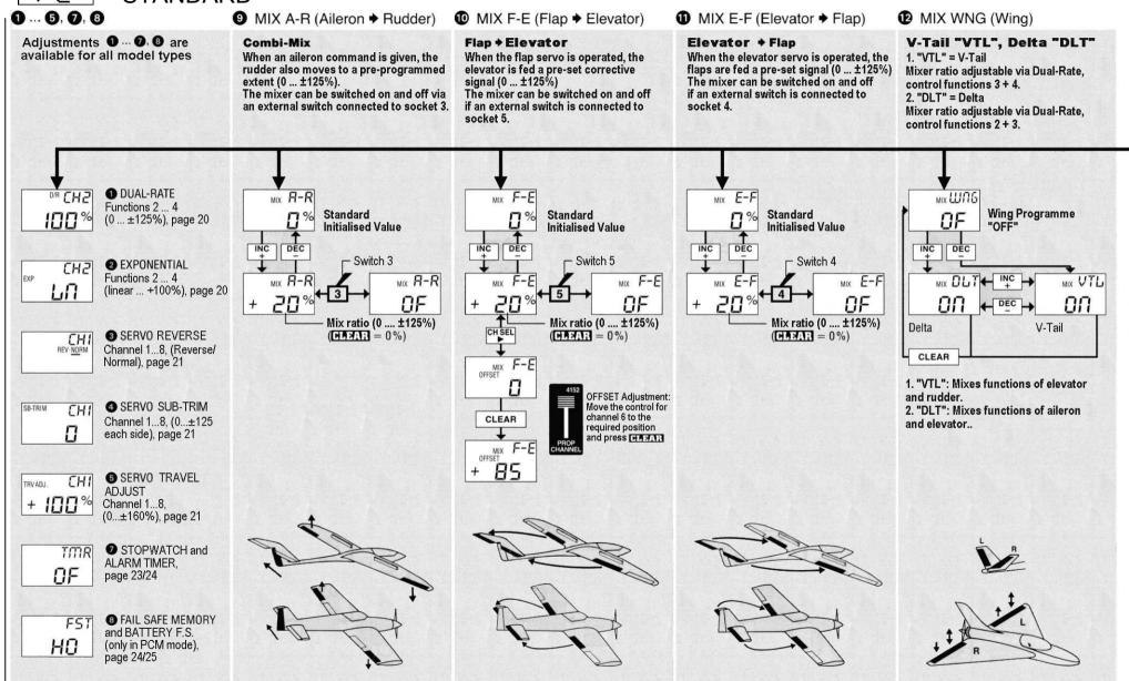
All mixer data can be reset to 0 by pressing the CLEAR button, i.e. turned off. When the display shows "OF" the external switch controlling the mixer is switched off.
