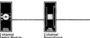
2 channel Switch Module with long arm Part No. 4151 with short arm Part No. 4151.1 2 channel Proportional Module Part No. **4152**
